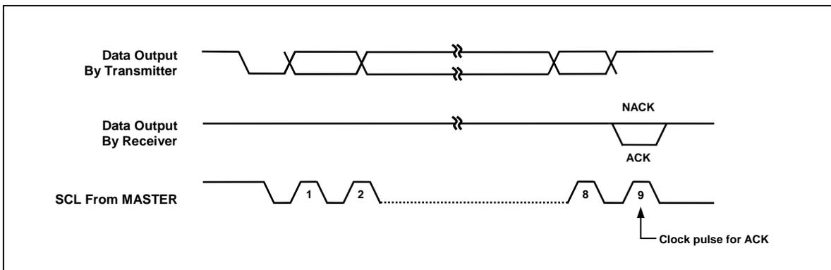
Figure 8 Acknowledge on the I<sup>2</sup>C-Bus
