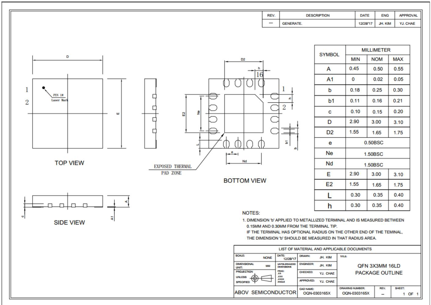
Figure 3 16-pin QFN Package
