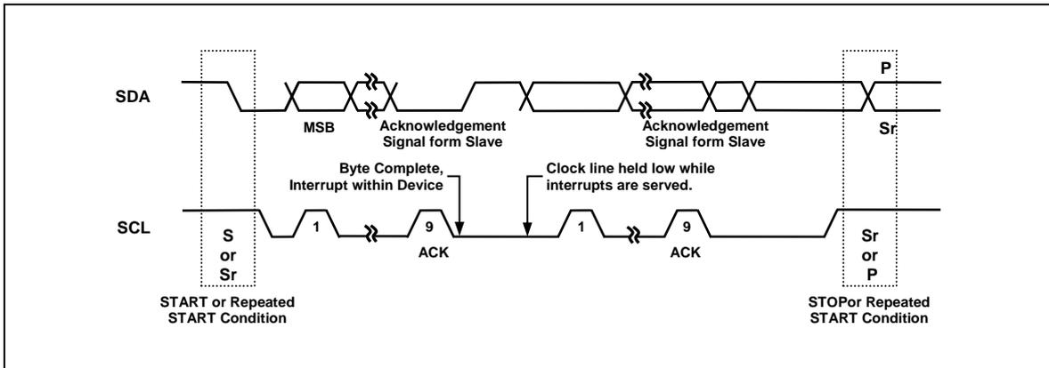
Figure 7 Data Transfer on the I<sup>2</sup>C-Bus
