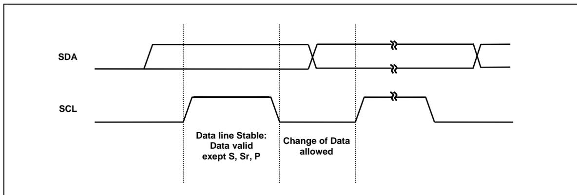
Figure 5 Bit Transfer on the I<sup>2</sup>C-Bus
