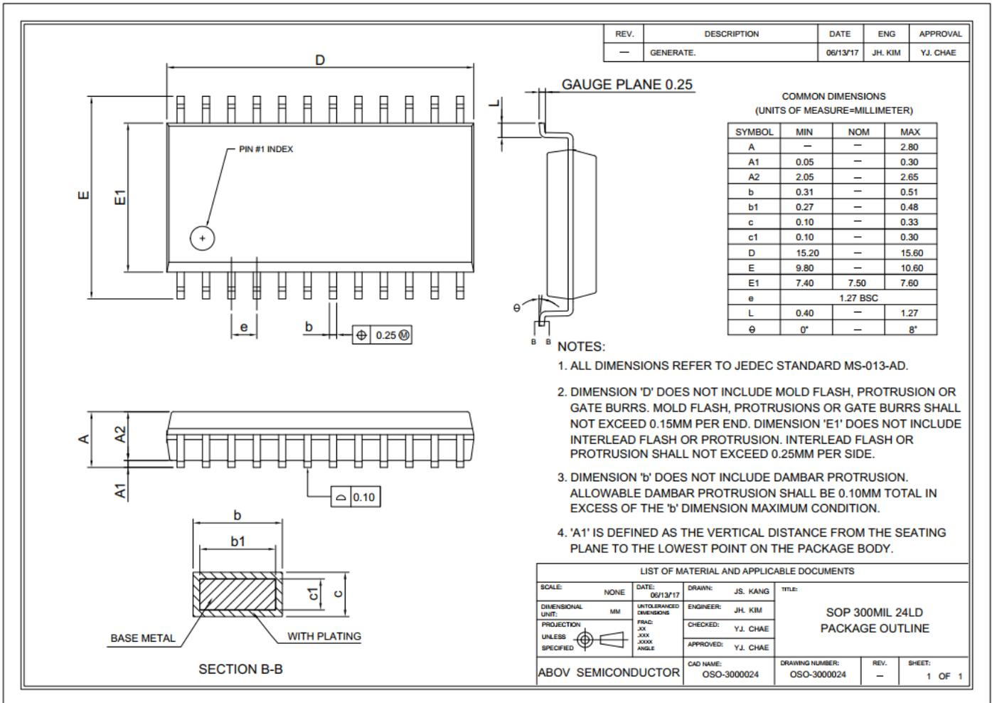
Figure 4 24-pin SOP Package
