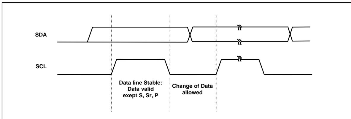
Figure 5 Bit Transfer on the I<sup>2</sup>C-Bus
