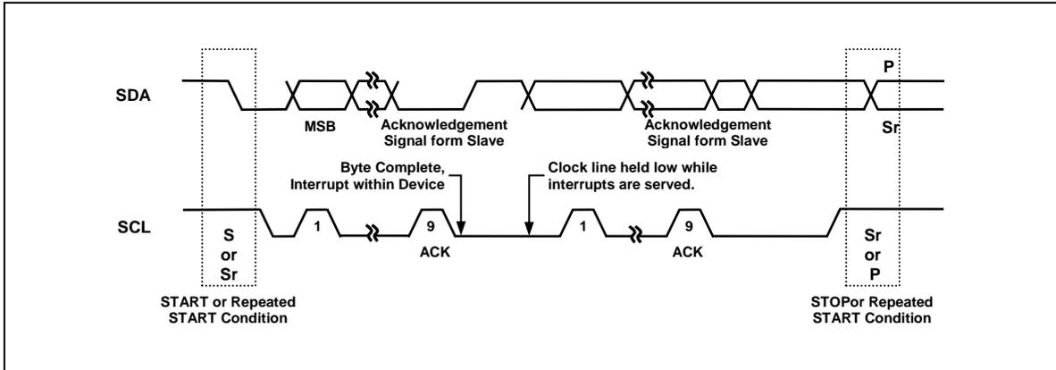
Figure 7 Data Transfer on the I<sup>2</sup>C-Bus
