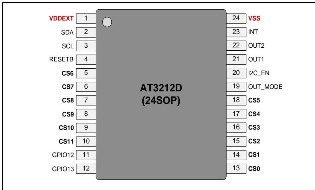
Figure 2 24-SOP Pin Assignment
