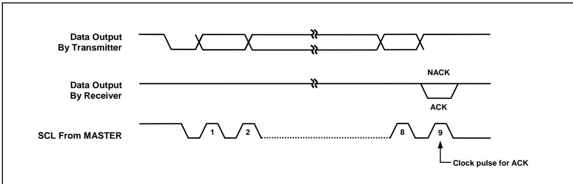
Figure 8 Acknowledge on the I<sup>2</sup>C-Bus
