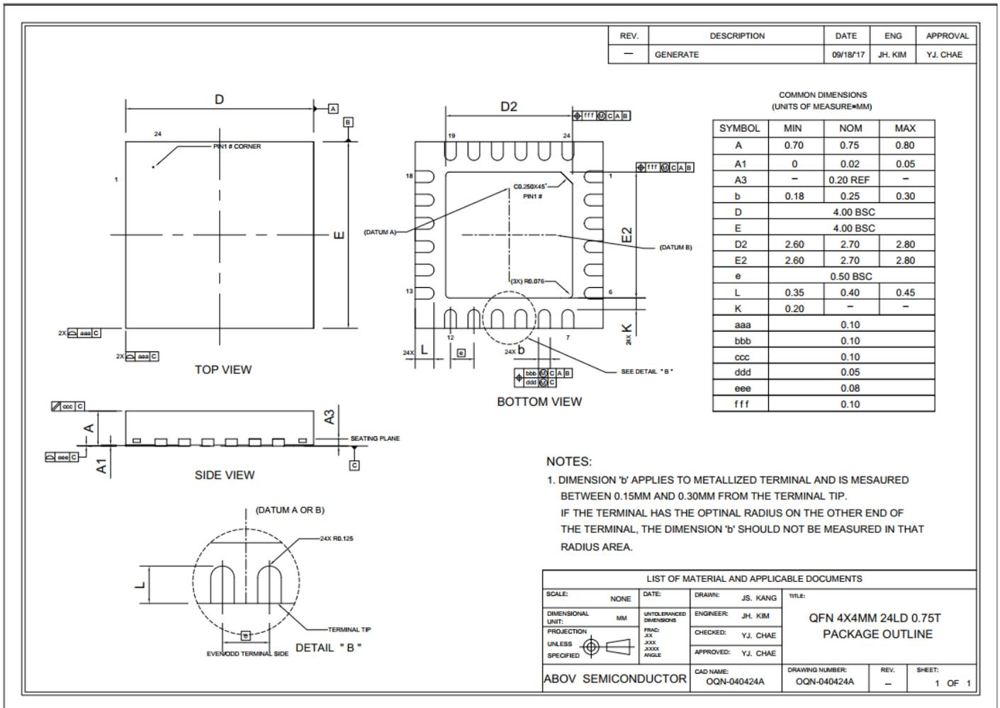
Figure 3 24-pin QFN Package
